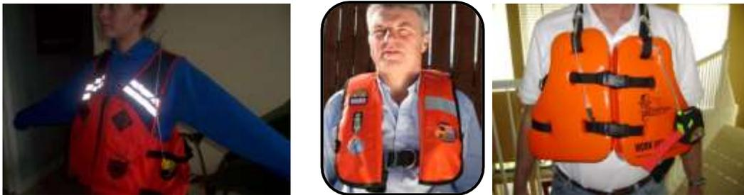
Normally, companies like Great Lake Dredge would simply use industrial VELCRO and fasten the alert to the vest and use Velcro straps or electrical tie wraps to create eyelets to string the lanyard antenna up and around the shoulders. In addition a protective pouch with a belt loop makes integration easier.
